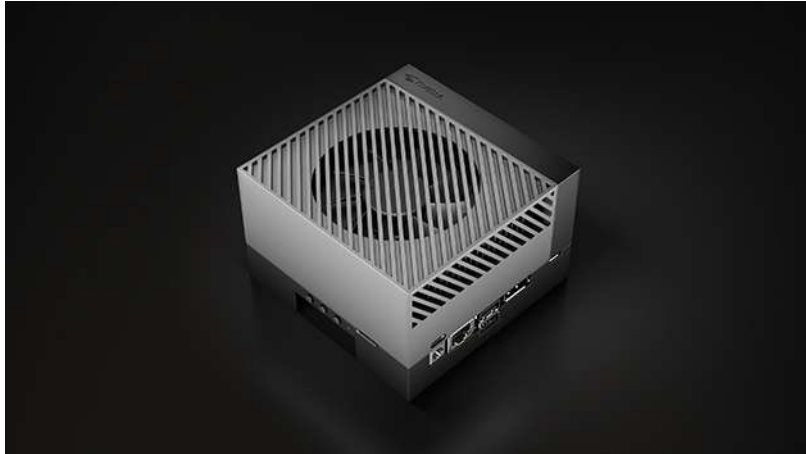
Figure A.5: Jetson AGX Orin Developer Kit used in the ARP laboratory.
